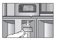
Pull the rubber disc top, down and out.
